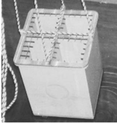
Fig. 4 Dismantled core flame and cut upper grid
