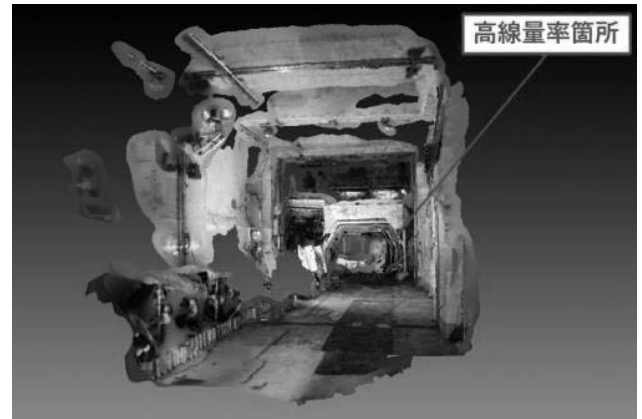
Fig. 7 An image of the hotspot measured using the Compton camera is drawn on the 3D structural model created via photogrammetry.
