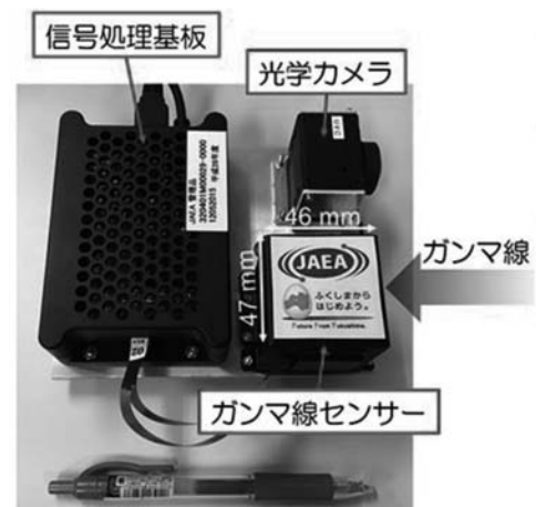
Fig. 1 A compact Compton camera composed of a gamma-ray sensor, signal-processing unit and an optical camera
